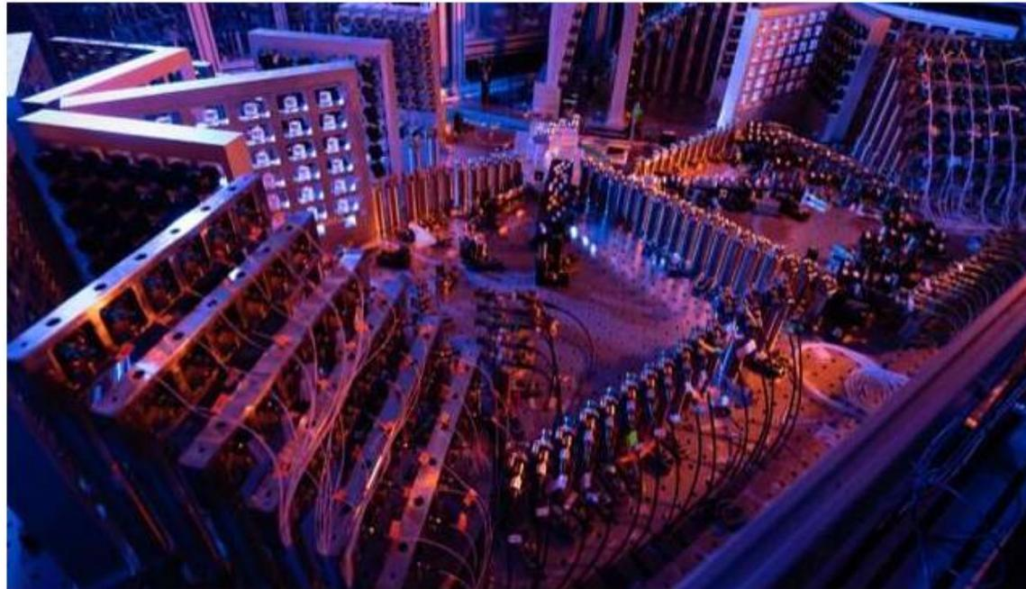
The Pan team's optical quantum computer uses a 144-mode interferometer to solve a Gaussian boson ...
